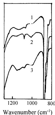
Figure 1 FTIR spectra of CaCO 3 surfaces: (1) HDPE/CaCO 3 (untreated), (2) HDPE/CaCO 3 (NDZ-treated), and (3) HDPE/CaCO 3 (NDZ-ON330-treated).
